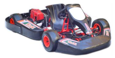
Chassis All 25mm tube Wheelbase 770mm Rear Axle 25mm solid
