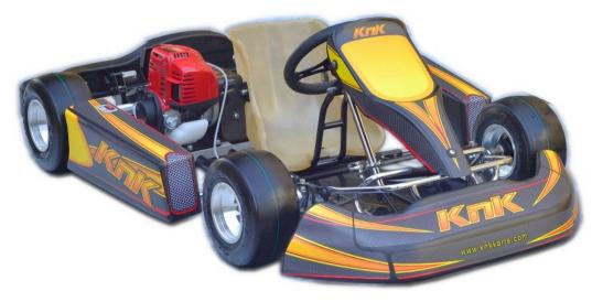
Chassis All 25mm tube Wheelbase 700mm 30mm hollow Rear Axle
